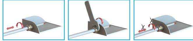
4. Do not pull or rotate cable after insertion if no adhesive copper tape is used (2b). Otherwise cable gland and shielding could be damaged.
