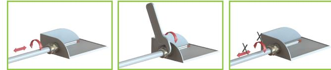
4. As long as the cap is not tightened, you can easily pull push or rotate the cable.
