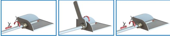
4. Do not pull or rotate cable after insertion. In doing so cable gland and shielding will be damaged.
