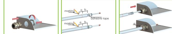
1. Install cable gland to the enclosure with the indicated "torque body". In order to increase contact quality EMC locknut utilization is recommended.
