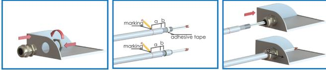
1. Install cable gland to the enclosure with the indicated "torque body". In order to increase contact quality EMC locknut utilization is recommended.
